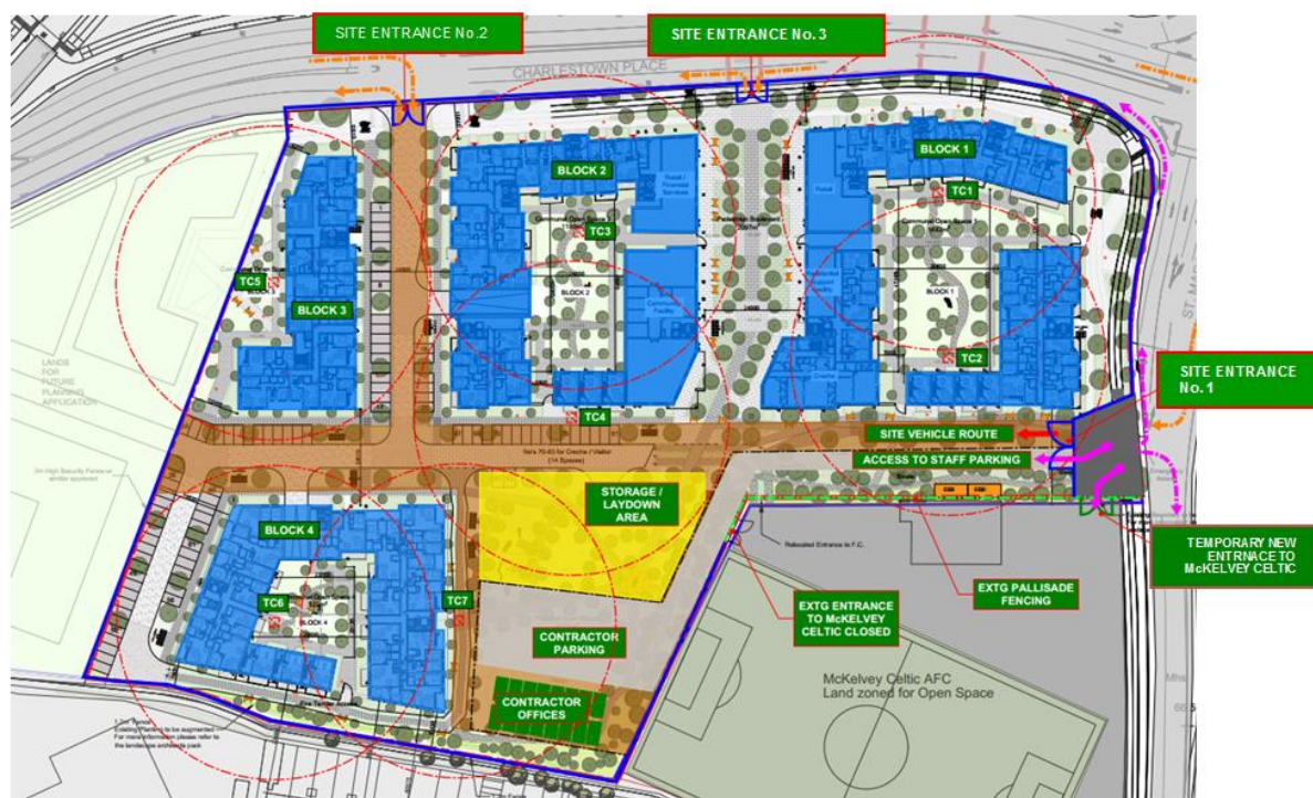
Figure 10.2 Construction site access
