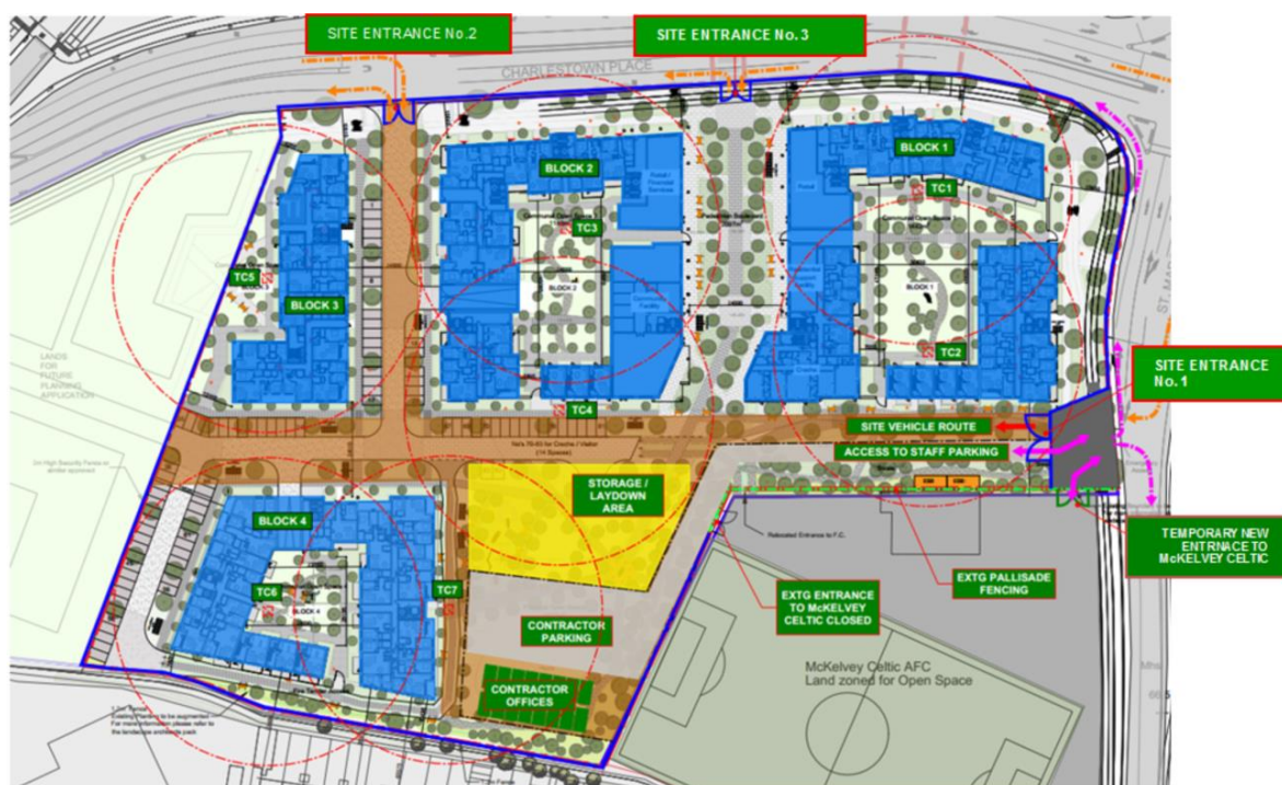
Figure 11.5 Proposed Construction Access Layout
